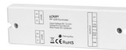
cod. LC9201 INPUT: 12-24VDC OUTPUT: 12-24VDC I MAX INPUT: 15A I MAX OUTPUT: 5A x 3 CH MAX LOAD: 3x60W @ 12V (TOT 180W) 3x120W @ 24V (360W) 434MHZ/868MHZ TA: -20°C +50°C
