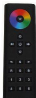
cod. LC2819 RADIO COMANDO SEI ZONE RF REMOTE CONTROL OPERATION VOLTAGE: 3x1,5V AAA (BATTERY) OPERATION FREQUENCY: 434MHZ / 868MHZ SIZE: 48 x 140 x 16MM TA: -20°C <> +40°C
