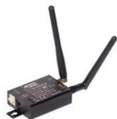
cod. LC2818WITR CONVERTITORE WI-FI / RF WI-FI / RF CONVERTER POWER SUPPLY: 9-12VDC (NON INCL.) WI-FI <> RF 434MHZ/868MHZ TA: -20°C <> +40°C
