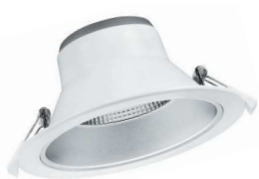
EXAL-LED 35 CRI>90 ELITE DALI / PUSH 220 ÷ 240 Vac / 35W / UGR<19 / CRI≥90 / SDCM 3 / Ta -15°...+45°
