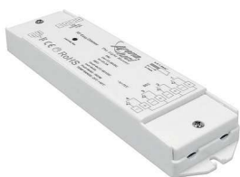
cod. LC1009FA INTERFACCIA RICEVITORE RGB / RGBW RGB / RGBW INTERFACE RECEIVER INPUT: 12-36VDC OUTPUT: 12-36VDC I MAX INPUT: 20A I MAX OUTPUT: 5A x 4 CANALI MAX LOAD: 4x60W @ 12V 4x120W @ 24V - 4x180W @ 36V SIZE: 46 x 178 x 18MM TA: -20°C +50°C
